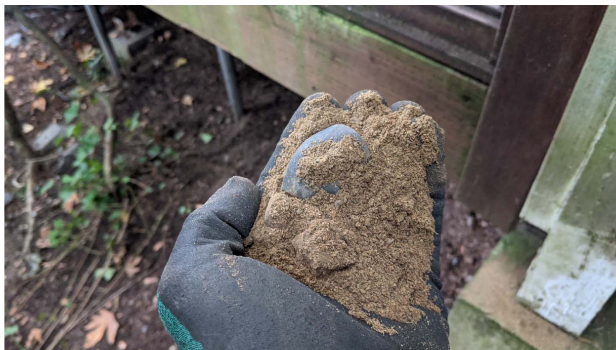
Plate 2: Cuttings from about 6 feet below surface in HB-2.
